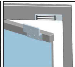
Demonstration of ZL Bracket Installation
